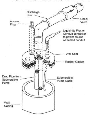
**Well Seal:** A properly sized well seal must be installed so as to provide a watertight seal between the casing and drop pipe.
